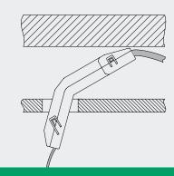
5. Clamp the light to the connection cable 6. Align and hold the tension springs upwards
